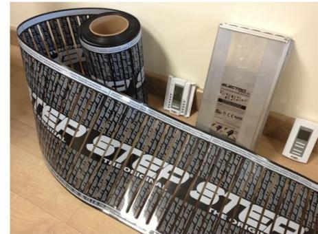
Another radiant heating option utilizes electric cables and flexible heating films to convert electric power into heat. Such systems require a thermal mass or an air gap to distribute the heat. The power generated is fixed and is controlled by on/off thermostats and floor sensors, creating differential temperature changes in the floor. Systems such as these require 11 – 12 watts per ft<sup>2</sup> of flooring.
