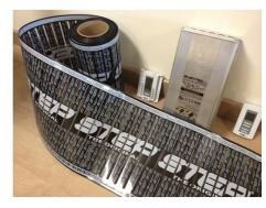
Another radiant heating option utilizes electric cables and flexible heating films to convert electric power into heat. Such systems require a thermal mass or an air gap to distribute the heat. The power generated is fixed and is controlled by on/off thermostats and floor sensors, creating differential temperature changes in the floor. Systems such as these require 11 - 12 watts per ft<sup>2</sup> of flooring.
