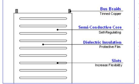
The EP-23-22W-24V STEP® Heating Element is a patented lowvoltage, strong, thin and flat heater. The heating element is constructed of two parallel bus braids embedded in a semi-conductive polymeric material.
