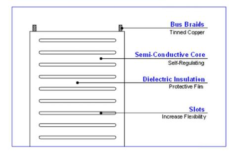
The EP-30-70W-24V STEP® Heating Element is a patented low-voltage, strong, thin and flat heater. The heating element is constructed of two parallel bus braids embedded in a semi-conductive polymeric material.
