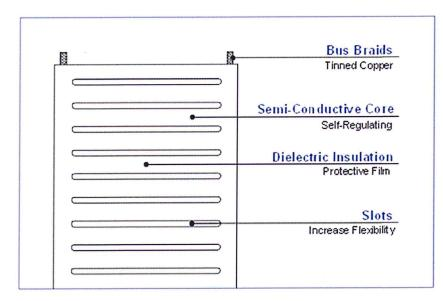
The EP-30-29W-24V STEP® Heating Element is a patented low-voltage, strong, thin and flat heater. The heating element is constructed of two parallel bus braids embedded in a semi-conductive polymeric material.
